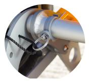
The wheels are mounted on axes and are entirely removable. Then, they are easily assembled thanks to the pre-mounted split pin.
